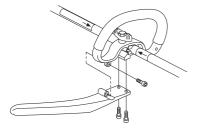
Now adjust the trimmer to give a comfortable working position. Tighten the bolt/knob.
